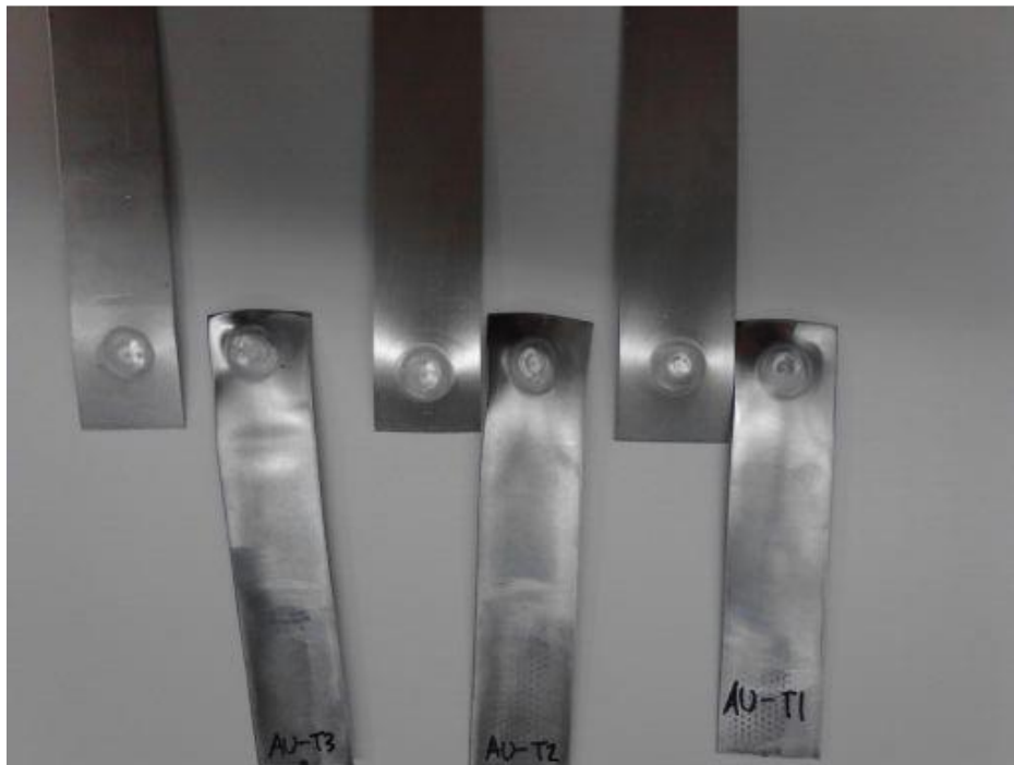
Figure 14: scraped shoulder plunge tensile samples after failure
