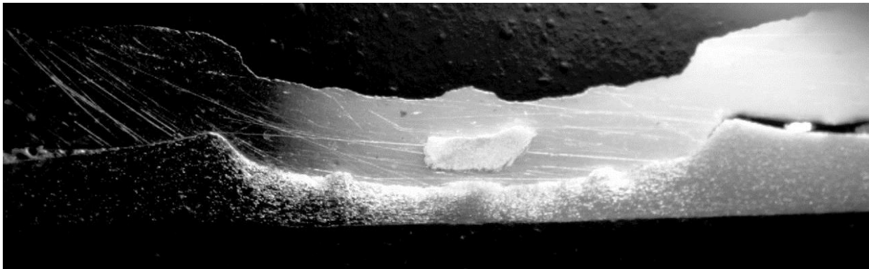
Figure 8: FSSW pin plunge made with scraped steel
