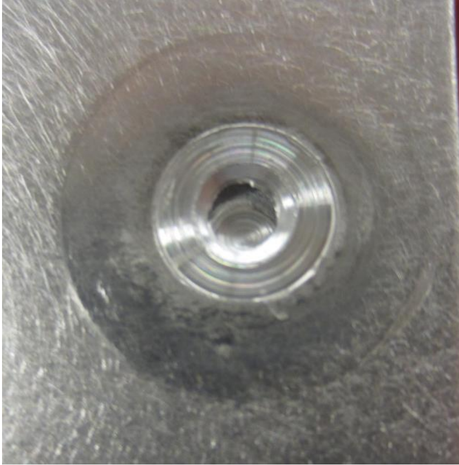
Figure 21: Close up of pin plunge sequence with uncoated steel tensile sample failure mode
