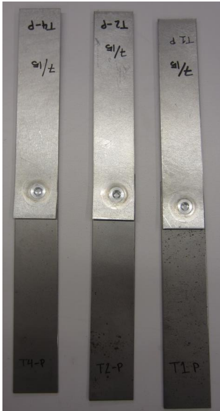
Figure 20: Uncoated pin plunge tensile samples after testing
